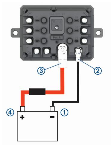
2 Connect the small ring end of the ground wire to the **GND** terminal (2) on the device.
