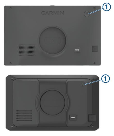
• To put the device in power saving mode, press the power key while the device is on. While in power saving mode, the screen is off and the device uses very little power, but it can wake instantly for use.
