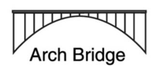
An arch bridge uses its semi-circular "arch" shape to distribute the force of compression by spreading the weight outward.
