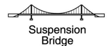
A suspension bridge suspends the deck by cables hung from towers. Compression tension is transferred from the cables to the towers to the ground.
