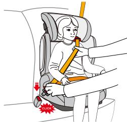
Pull out the vehicle seat belt and guide it in the front of your child to the vehicle seat buckle. Engage the buckle tongue in the vehicle seat buckle. CLICK!
