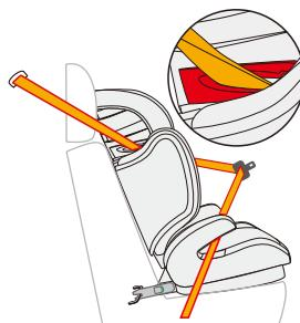
**⚠** An unoccupied child safety seat should still be fastened
