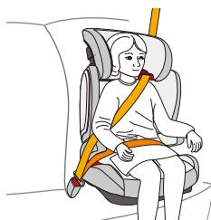
Divide the lap belt section and the diagonal belt section on the side of the vehicle buckle. The lap belt section shall be placed under the armrest into the red belt guide of the seat cushion. The diagonal belt section shall be placed above the armrest.
