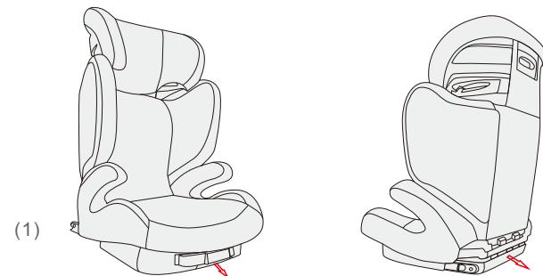
Pull to unlock(1) and simultaneously pull and release the connector block(2).
