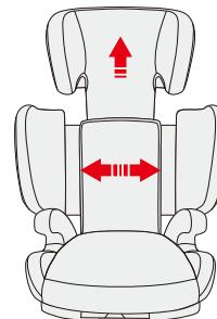
You can now adjust the released headrest to the desired height. As soon as you have let go of the adjustment handle, the headrest will engage.
