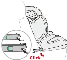
For the Stability fix model lock on the two stability fix connectors to the anchorages in your car seat.
