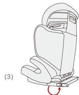
Rotate the connectors into position.
