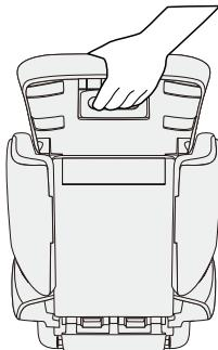
Grasp the adjustment handle by the back of the headrest and pull it up wards slightly. The headrest is now released.
