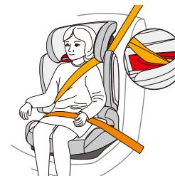
Insert the lap belt section on the other side of the seat base into the red belt guide as well.
