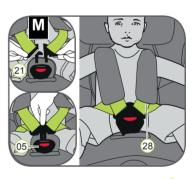
19. Guide the two buckle latches 21 together and engage them before putting them into the harness buckle 05 - this should make a clicking noise.
