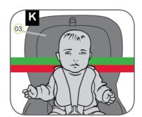
A correctly adjusted headrest (3) ensures optimal protection for your child in the safety seat:
