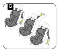
Hook the snap hook (26) into the Top Tether anchoring point recommended in your vehicle owner's guide.
