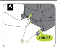
Pull the grey fabric loop 16 to pull out both locking arms 17 until you hear a clicking sound which indicates they are fully engaged.
