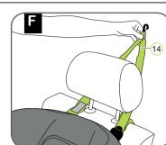
Guide the Top Tether (4) on the left and right-hand sides past the headrest.
