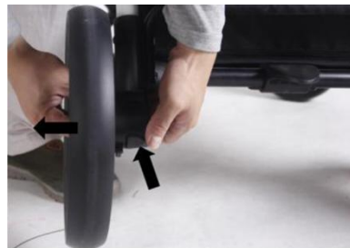
10.3 Removal of rear wheels Pull the metal plate up, in order to remove the rear wheels.
