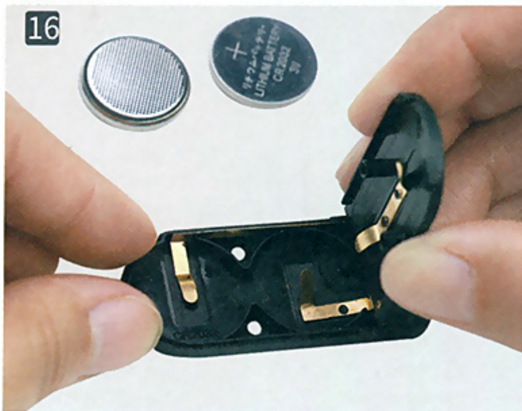
Put battery in the box.(Pay attention to the Positive & Negative)
