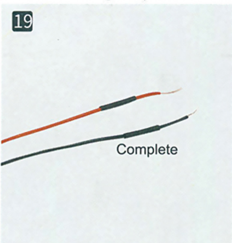
Cut off 2pcs shrinkable tubes(20mm) and cover the wire.
