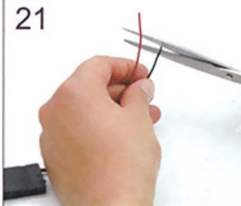
Peel off the rubber (12mm)
