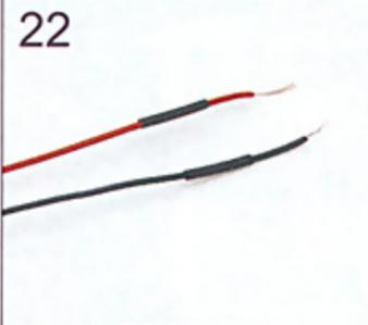
Cut off 2pcs shrink tube (20mm) and cover the wire.
