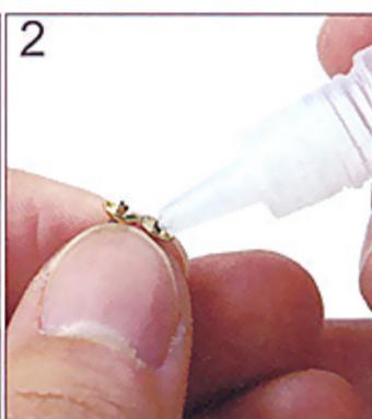
Put the ends of U shape metal wire through the receptacle and fix with glue.
