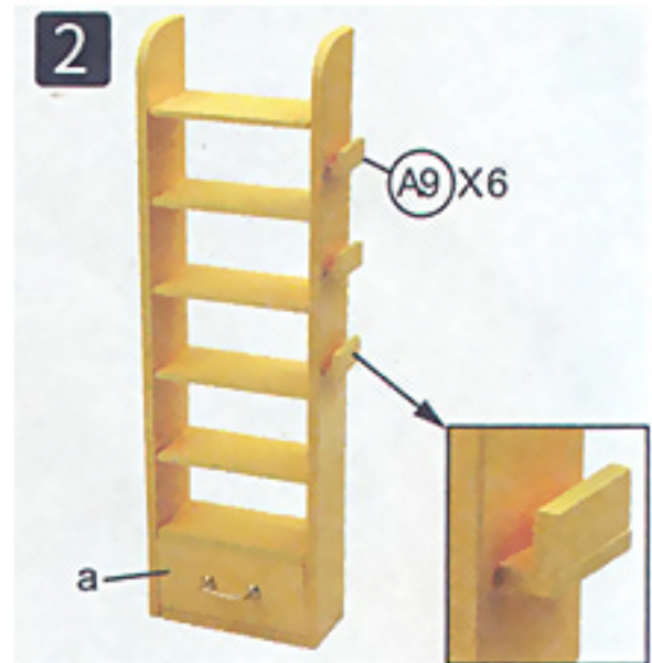
a is same with the step 1 & step 2 in Cabinet 1. Glue a with A9.
