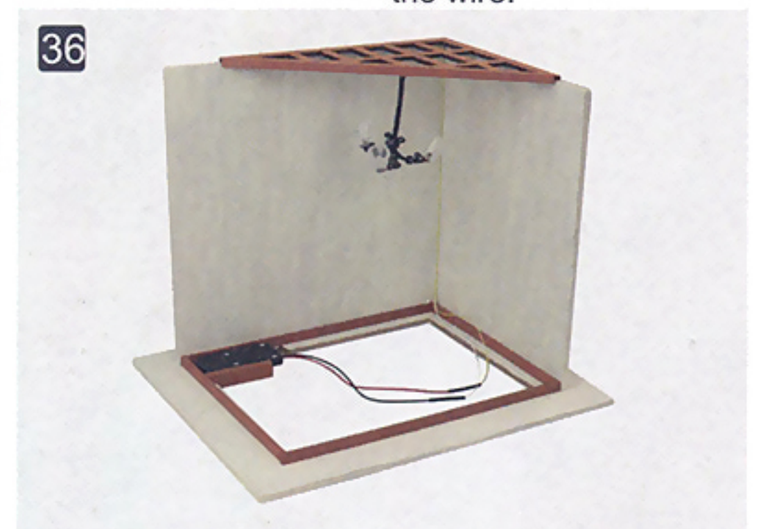
36 Put the battery in the correct position. Switch downward. Attention: Do not glue in case of change battery.
