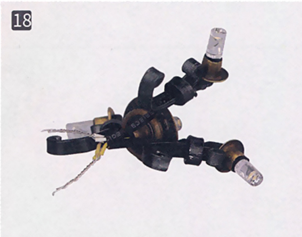
Combine step 17 with step 11. Twine the same color wire together.(Test the lamp)
