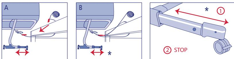
\*Note: For easier installation, keep the cot slightly separated from the adult bed and then move it closer by tightening the straps.
