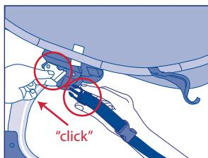
6) Pass the free end of the strap underneath the structure of the adult bed (A) and wrap it round to fasten the free end of the red clasp with the red clasp positioned closest to the BABYSIDE cot (B).
