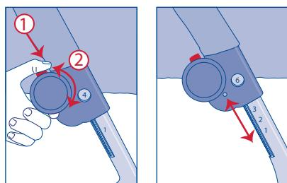
**\*Note:** The co-sleeping cot can be tilted with a maximum difference of 2 positions between one side and the other. The baby's head should always be in the highest part of the cot.
