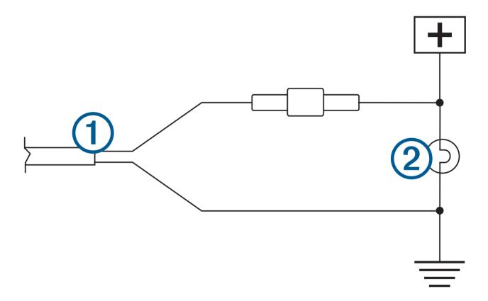
**NOTE:** Connecting the transmitter to an always-on 12 to 24 VDC source, such as a running lamp, instead of a reverse lamp requires you to manually switch power to the transmitter. The transmitter may drain your vehicle battery if it is left on.
