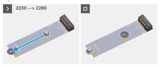
The following image indicates the location of the M.2280 solid-state drive and provides a visual representation of the installation procedure.
