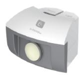
Light sensor uses the silicon photoelectric cell as the sensing element; it can convert the light ntensity into a voltage signal, keeping a direct proportion. For the sensor, the effective light spectrum is in the range of 380nm to 730nm, it is an ideal intensity sensor for visible light.
