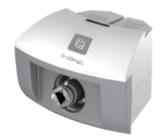
The probe of the dissolved oxygen sensor works as per the polarogram measurement principle. The probe electrode composes of the anode, cathode and membrane. When is usage, immerse the electrode into the solution and apply the electric potential between the anode and the cathode to generate the electrochemical reaction; Dissolved oxygen sensor also can be used for measuring oxygen content in gas.
