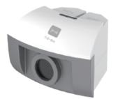
Motion sensor is a sonar equipment emitting ultrasonic pulse, it receives signal through the reflection of object, and then measure the time T when the high frequency sound wave goes around between the object and sensor; in accordance with the speed of sound in air, i.e. V, it can calculate the distance between the object and the sensor, i.e.:  $d=V^{*}T/2$ .
