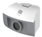
Motion sensor is a sonar equipment emitting ultrasonic pulse, it receives signal through the reflection of object, and then measure the time T when the high frequency sound wave goes around between the object and sensor; in accordance with the speed of sound in air, i.e. V, it can calculate the distance between the object and the sensor, i.e.:  $d=V^{*}T/2$ .
