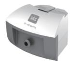
Absolute pressure sensor is used to measure the absolute pressure of air, it is connected with the exterior air under measurement by the front luer, whereas the luer and the sealed vacuum reference cavity inside the sensor forms a pressure difference; after the pressure difference is converted into a voltage signal, its output voltage and absolute pressure to be proportional.
