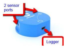
The Splitter fits into one of the mini USB 8 ports located on the side of the data logger. After inserting the splitter two devices can now be plugged into the port.
