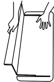
Fold the Reinforcement section to a 90° angle.
