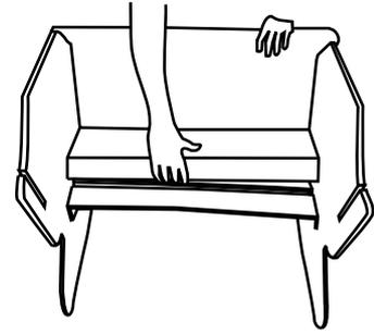
Lower Part B into Part A, be sure to lower evenly on both sides. Hold the Reinforcement Section so it does not drop below the Middle Section. Insert the Reinforcement section into the groove in the connecting segment.
