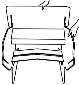
Align the slits on Part B with the slits on the Rocking Sides.
