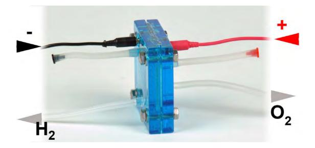
When the fuel cell is operated in regenerative mode, the anode for the electricity production mode (fuel cell mode) becomes the cathode in the hydrogen generation mode (reverse fuel cell mode), and vice versa.
