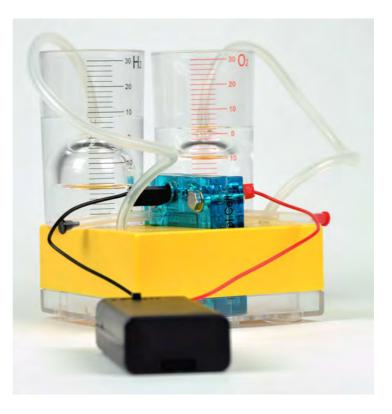
You should produce a volume of about 20 ml of Hydrogen or more. Upon that remove the cables of the battery pack generator from the Electrolyzer.
