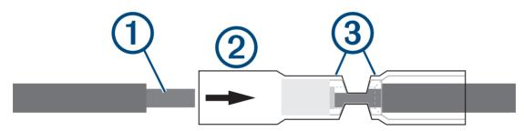
3 Insert one bare wire into one end of the heat-shrink crimp connector ②. The bare wires are not secure until they are crimped and sealed.
