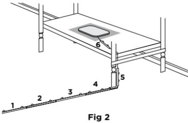
Use the crib leg by the wall closest to the Nursery Unit (**Fig 1**). In cases where the Nursery Unit is across the room, use the leg closest to the Nursery Unit to position the covered wire (**Fig 2**). It is always preferable that the covered cord run along a wall.
