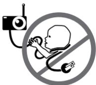
Keep adapter cords out of the reach of children (more than 1 m away). **NEVER** use Sensor Pad without the protective cord covering. Check protective cord covering before each
